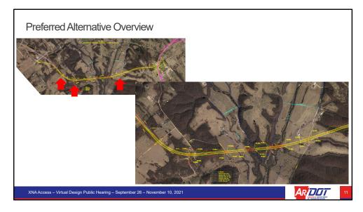
Beginning at the trumpet interchange and proceeding north, the XNA Access Highway will be a four-lane divided highway for 2.5 miles. The highway will be fully access controlled, meaning there will be no driveway or local road connections, and access will only be allowed at the interchanges serving Hwy. 612 and Hwy. 264.
