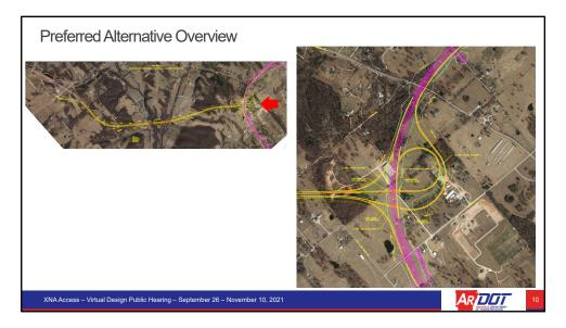
The trumpet interchange on the southern end would be designed to connect to the future location of Hwy. 612 between Hwy. 112 and Hwy. 412, which is planned to be built prior to the construction of the new XNA Access Highway. This future interchange location was identified based on interchange spacing requirements by FHWA and consideration of environmental impacts.
