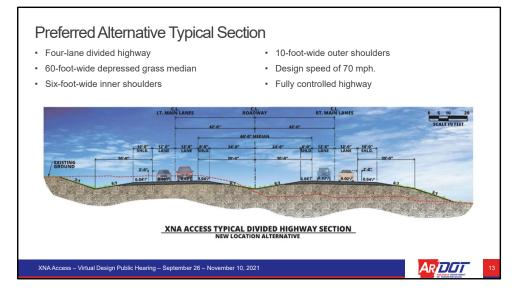
Concerning the roadway and its appearance, the typical section would consist of a four-lane divided highway with a 60-foot-wide depressed grass median, six-foot-wide inner shoulders, and 10-foot-wide outer shoulders. The design speed would be 70 mph. The design speed will be reduced to 55 mph in the two-lane transition section, nearing Highway 264.
